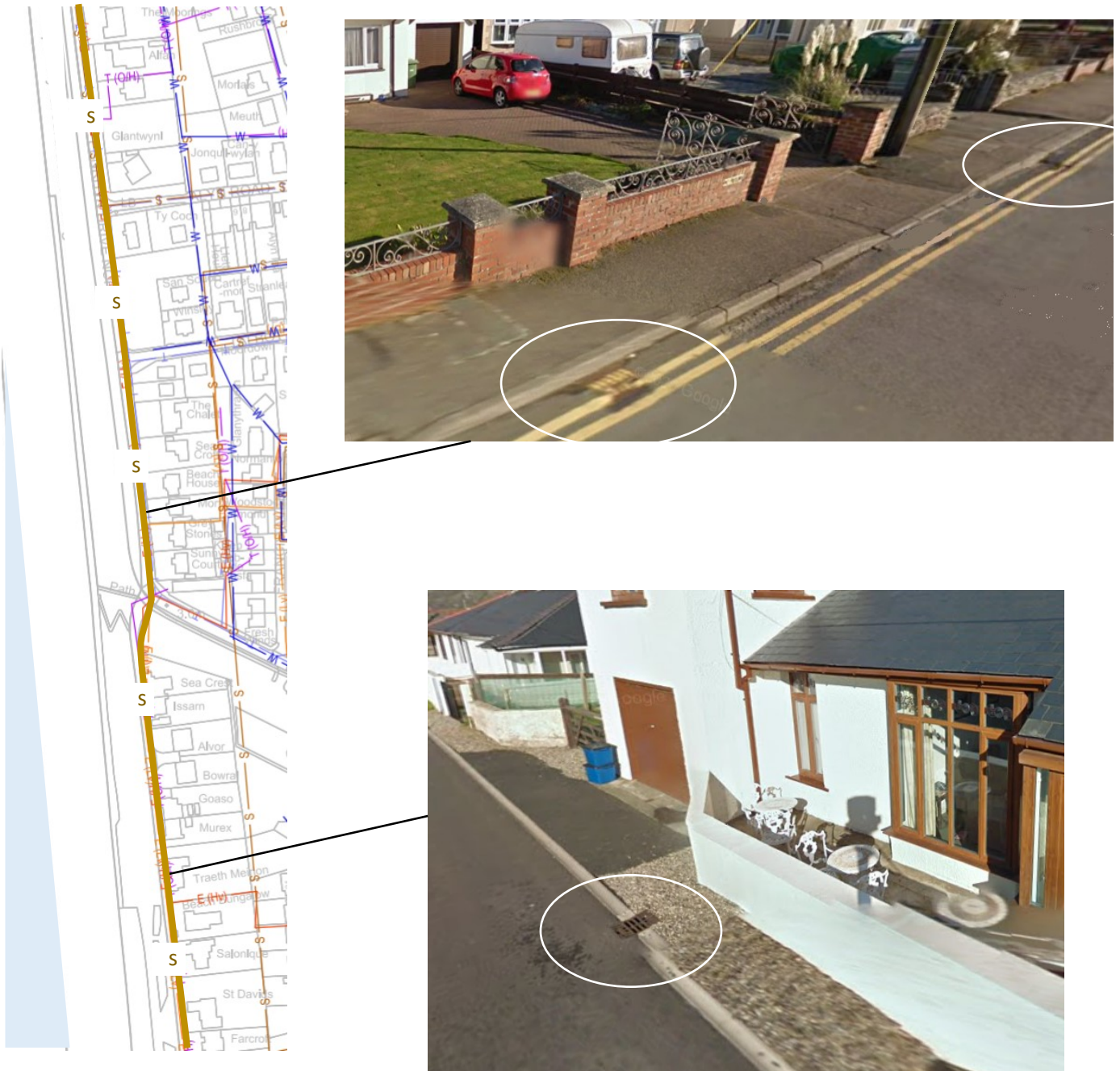
Figure 35: (left) Utilities map indicating the location of a buried sewer along Penrhyn Drive (after Black and Veatch, 2012). (right) Roadside drainage grids in front of properties in Penrhyn Drive.
