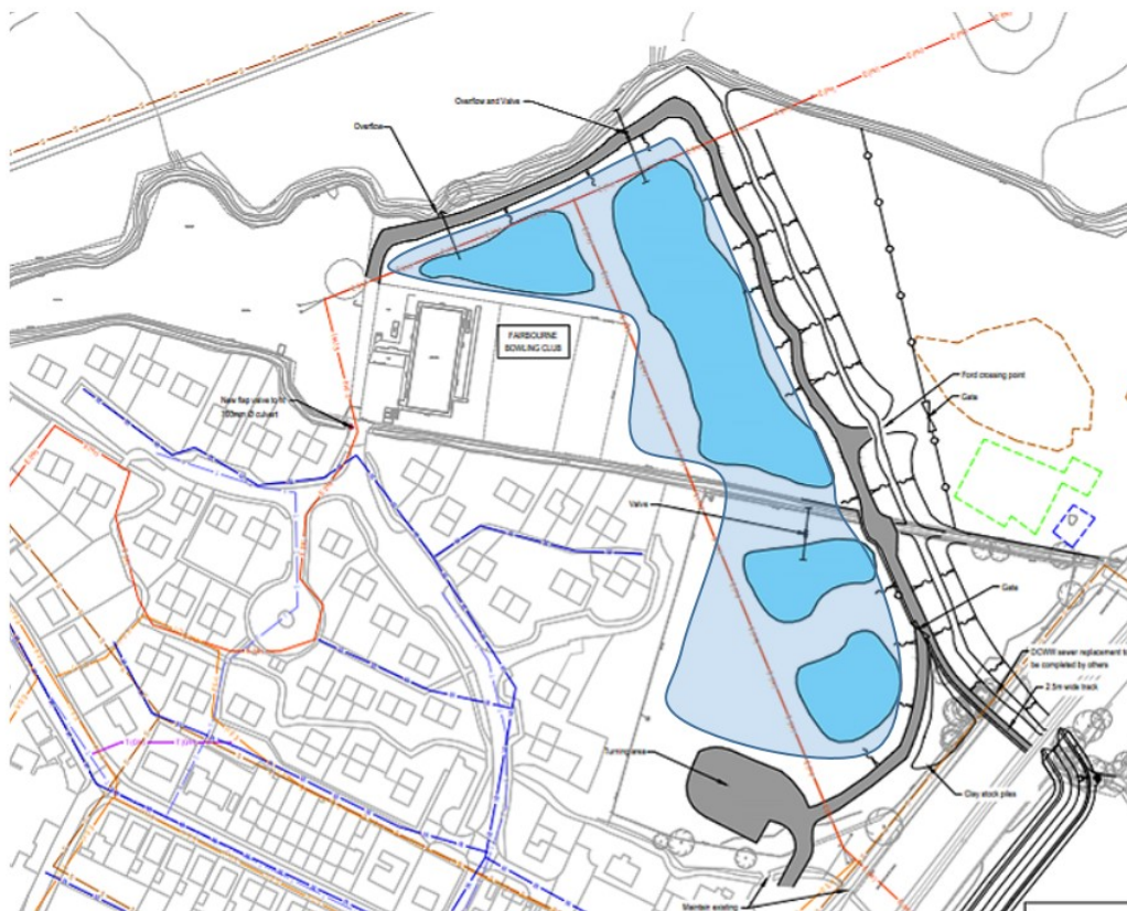
Figure 74: Available area for excavation of clay and creation of a flood water retention pond (after Black and Veatch, 2012).
